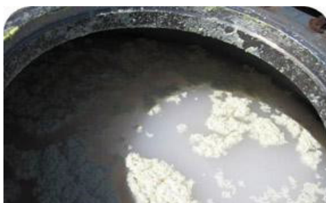
Image 6: Example of filter blockage and tank residues known as a reverse emulsion resulting from incorrect mixing procedure (Source: SACOA)
