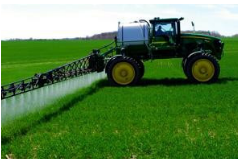
Image 1: Modern spray equipment is designed for efficient coverage of large areas – however care should be taken with speed of tank filling and mixing (Source: SACOA)
